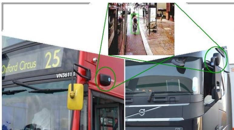
Fig. 2.15. CycleEye – Collision Avoidance Sursa: Fusion Processing, 2014
